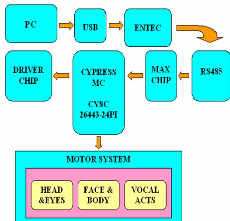
Fig 5.1 Hardware and Software Interface of SSU-1
